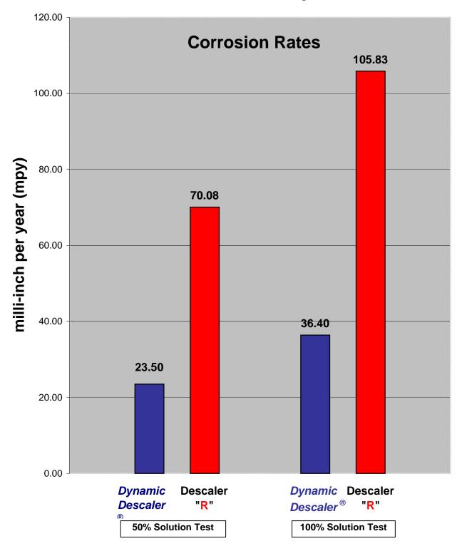
Results of corrosion tests\* done on Dynamic Descaler and another leading descaler by an independent lab in October 2006.
